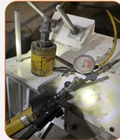
Pull tested anchor bolts to 22 tonnes for 15 minutes
